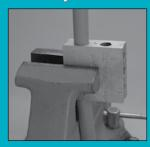
Using the Parker VBS or VBL vise block, place hose in proper hole of the vise block and then clamp in a bench vise. Ensure enough hose extends from the vise block to install socket.
