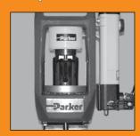
Assemble hose - Insert hose and fitting from bottom of crimper and up through die set. Position fitting so bottom of fitting skirt rests on die step (PARKÄLIGN® feature).
