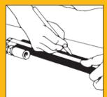
Measure hose to length - Measure and mark the length that the hoses are to be separated (commonly referred to as Splitback Length).
