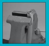
Place hex portion of socket into vise and tighten vise. Ensure socket extends past vise jaws enough to allow for installation of nipple.
