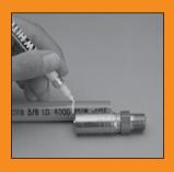
Insertion Depth – Mark hose end with proper insertion depth line. See Hose Fitting Insertion Values, pg. G-43 for insertion depths of fitting series that do not incorporate an insertion depth
