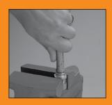
Push hose bore onto nipple to size tube and to aid in separating braid before assembling ferrule onto hose.
