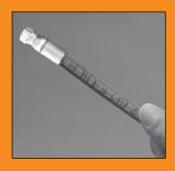
Inspect insertion depth mark at fitting ends. Insertion mark must be visible but not exceed 1/8" from end of crimped fitting shell.
