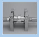
Loosen swaging bolts to release pressure on dies.
