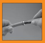
Using a tapered punch, push punch into end of sleeve and tube to set sleeve barbs into
