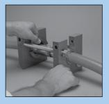
Insert both die halves around hose in each end of swager.
