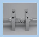
Remove die securing bolts and nuts. Then remove dies.
