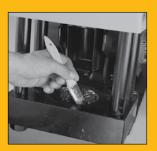
Using a premium, quality, lithium-base grease, apply a thin layer of grease on bowl of crimper base plate.
