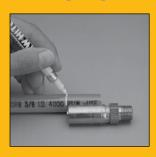
Insertion Depth – Shown is a 55 series fitting. See Hose Fitting Insertion Values, pg. G-43 for insertion depths of fitting series that do not incorporate an insertion depth. Mark hose end with proper insertion depth line.
