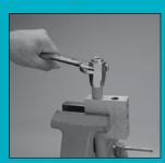
Using a wrench, screw socket onto hose counterclockwise until it bottoms. Ensure end of hose is against inside shoulder. Back off socket 1/4 turn clock-
