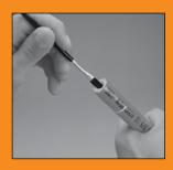
Lubrication (as required) -Using an SAE 20 weight lubricating oil, lightly lubricate inside of hose end.
