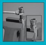
Using a wrench on the nipple hex, screw nipple into socket clockwise until nipple bottoms against socket shoulder.
