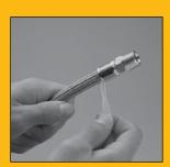
**Assemble hose – Push fitting** onto hose slightly and then remove tape. Continue pushing fitting onto hose until fitting reaches depth insertion mark.
