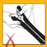
Figure 1 - Extreme care must be taken to avoid cutting through the cover of the hoses and thereby exposing the hose reinforcement. If this occurs, the hose assembly must be discarded.
