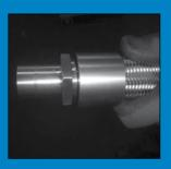
d. Pull collar out towards end of insert until at correct crimp position on insert of collar.
