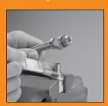
Using SAE 20 weight oil, lubricate nipple and socket threads. For stainless steel fittings use Parker ThreadMate™ or a molybdenum type lubricant.
