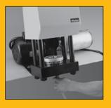
Assemble hose - Insert hose and fitting from bottom of crimper and up through die set. Position fitting so bottom of fitting skirt rests on die step (PARKALIGN® feature).
