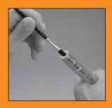
**Lubrication (as required) –**Using an SAE 20 weight lubricating oil, lightly lubricate inside of hose end.
