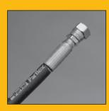
Inspect insertion depth mark at fitting ends. Insertion mark must be visible but not exceed 1/8" from end of crimped fitting shell.
