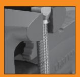
Remove assembly from vise and reposition with socket in vise jaws. Ensure socket extends beyond vise jaws far enough to allow nipple to be completely tightened.
