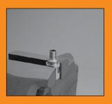
Mount nipple hex in vise. Ensure nipple end extends beyond vise jaws sufficiently to allow installation of hose.
