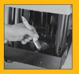
Grease frequently using a premium, quality, lithium-base grease. Apply a thin layer of grease on bowl of crimper base plate.
