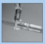
Measure swage diameter of each fitting at top, middle and bottom of shell. Take measurements at a minimum of three places around shell circumference. Verify swage diameter is within tolerances.
