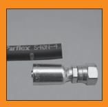
Insertion Depth - Shown is a 56 series fitting. Using Parflex Depth Insertion Block (part# TH9-1-56), mark the hose with the proper insertion depth line. On some fittings such as 55 Series, this depth is represented by a dashed or knurled line on the crimp shell.
