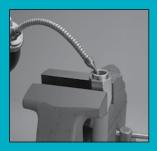
Using an SAE 20 weight lubricating oil, generously lubricate nipple and socket, threads and hose I.D.
