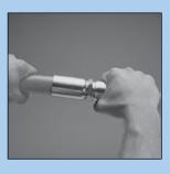
**Assemble hose –** Push each hose end into fitting to the depth insertion mark.
