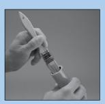
**Lubricate –** Using an SAE 20 weight oil, lightly lubricate inside of both hose ends.
