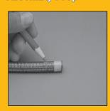
**Insertion Depth - Mark hose** end with proper insertion depth line. See Hose Fitting Insertion Values, pg. G-43 for insertion depths of fitting series that do not incorporate an insertion depth. For jacketed PTFE hoses, use a sharp knife and light pressure to cut back the cover at least the length of the insertion depth of the fitting.
