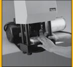
**Die Ring –** Place applicable die ring on top of die. Position ring so it is centered on die.
