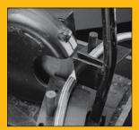
Using a power hose cutoff saw, cut hose squarely.
