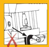
Figure 2 – The separation length must allow for the swaging or crimping operation without damaging the hose.
