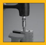
Using Parker VBS or VBL (vise blocks) and a rubber mallet, tap fitting onto hose until bottom of fitting shell is aligned with depth insertion mark.
