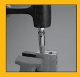
Using Parker VBS or VBL (vise blocks) and a rubber mallet, tap fitting onto hose until bottom of fitting shell is aligned with depth insertion mark.
