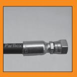
Assemble hose - Push hose into fitting all the way to depth insertion mark. (If fitting does not readily slide onto hose, perform the next step.)
