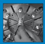
Crimp assembly only in Parker Approved adjustable crimper. Select correct die and crimp spec from Parker Crimp Source.
