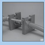
Install both die securing bolts with nuts positioned in opening of swager plates. Tighten die securing bolts 1/4 turn past finger tight.
