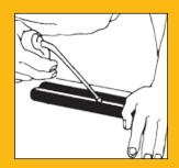
Lubricate - Lightly lubricate the web area between the hoses.
