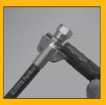
Measure crimp diameter of each fitting at top, middle and bottom of shell. Take measurements at a minimum of three places around shell circumference. Verify crimp diameter is within tolerances.
