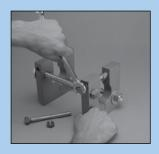
Remove both die securing bolts and nuts.
