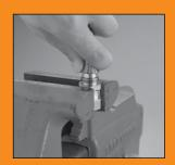
Assemble hose - Using a twisting motion, push hose over nipple until hose is seated against nipple chamfer.
