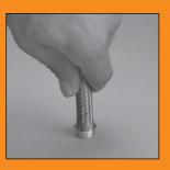
To complete positioning of sleeve, push hose end with sleeve against a solid flat
