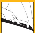
Cut Hose to Length - Press the multi-line hose assembly firmly and flat against the work surface with your free hand so that it does not move. Using a sharp utility knife, carefully draw the knife toward you with constant light to moderate pressure, and a smooth stroke. Multiple strokes will be necessary to separate the hoses.
