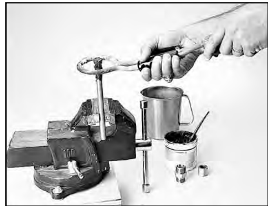
Fig. S22 – Multi-flame torch brazing
